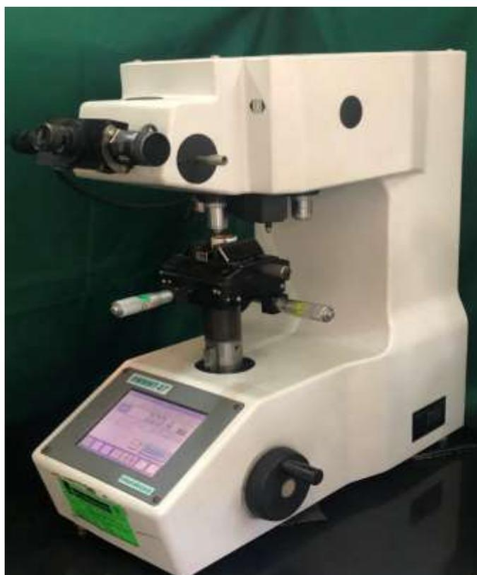
**Fig. 12: Microhardness tester - HMMT-XLE, Shimadzu, and Kyoto, Japan**
