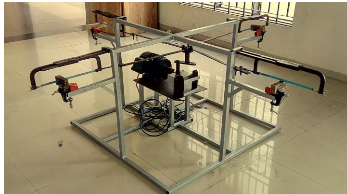
Fig. 3: Four-way hacksaw machine
