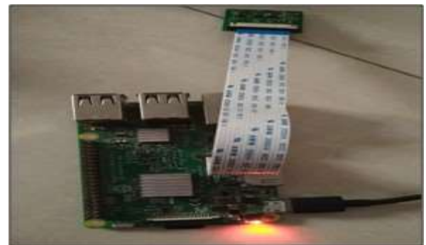
Fig. 2: Hardware implementation of video streaming
