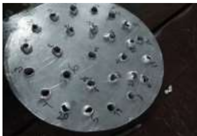
Fig. 18: Work piece after machining at dry condition without back up support with varying depth of cut
