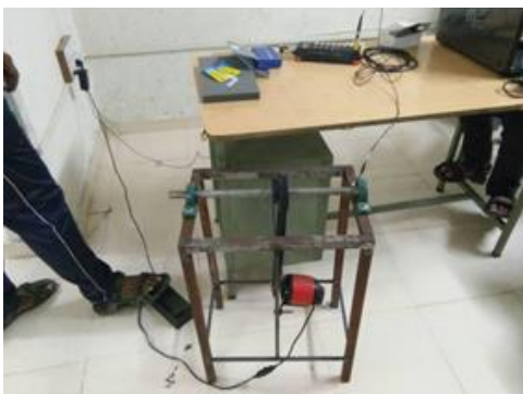
Fig. 18: Experimental Testing using FFT Analyzer
