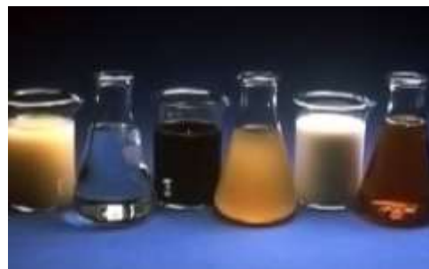
Fig 1: Liquid admixtures, from left to right: anti wash out admixture, shrinkage reducer, water reducer, foaming agent, corrosion inhibitor, and air-entraining admixture
