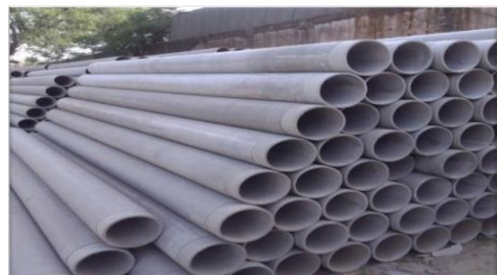
Fig. 3: Asbestos fiber reinforced concrete
