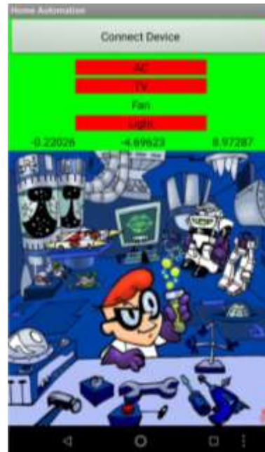
Fig. 10: Tilting left turns ON Fan and right tilt turns ON AC
