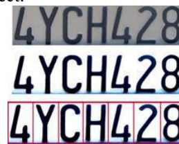
Fig. 1: Steps 2, 3, and 4: The license plate is normalized for brightness and contrast, and then the characters are segmented to be ready for OCR
