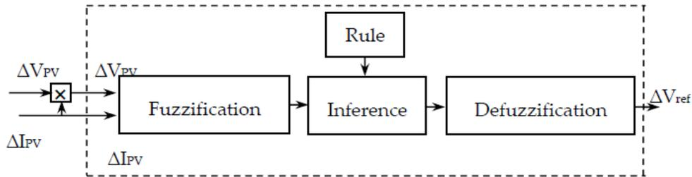
**Fig. 4: Diagram of a Fuzzy logic Controller**
