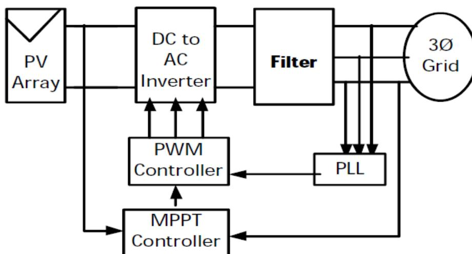
Fig. 1: Block diagram of the PV grid connected the inverter
