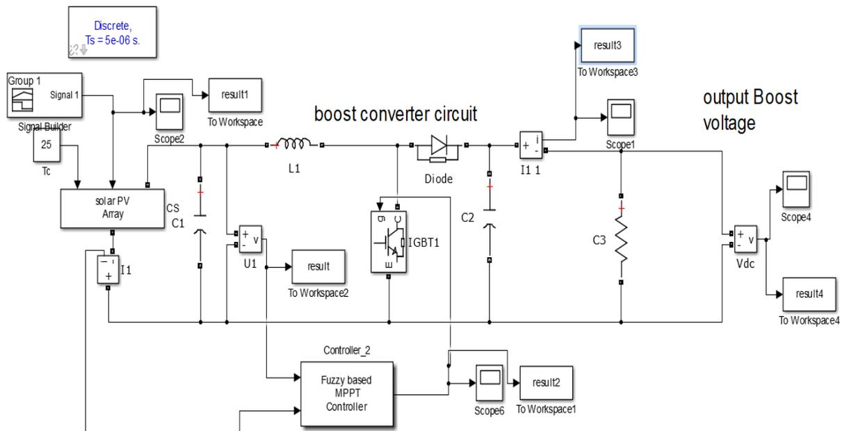
**Fig. 6: Simulink model of research work**
