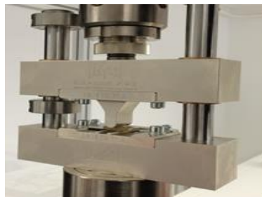
Fig. 8: Specimen under ILSS evaluation
