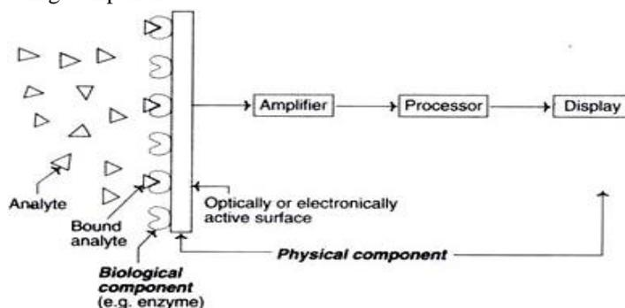
Fig. 1: A diagrammatic representation of a biosensor
