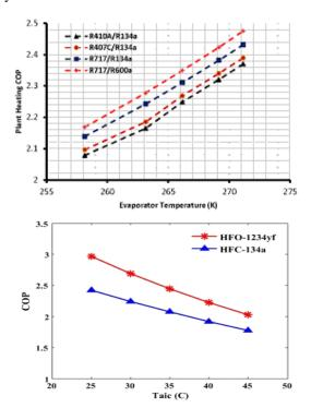
In the above figure, we can see the comparison in the cop of different refrigerants.
