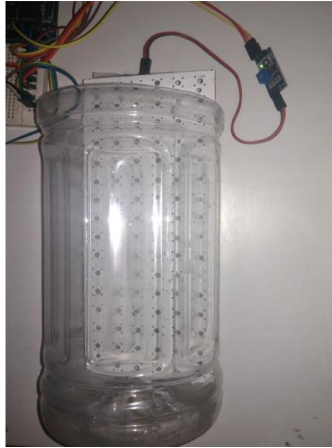
Fig. 7: Water level sensor with the container for the demo
