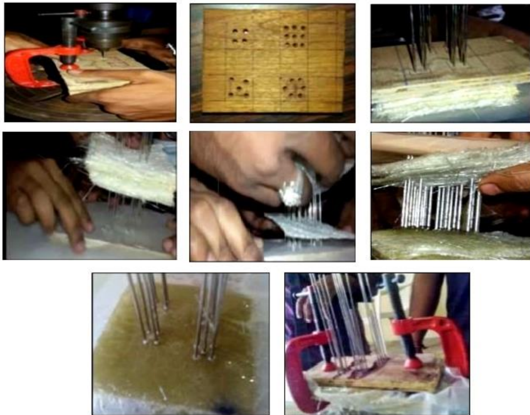
Fig. 1: Manufacturing of GFRP and S-GFRP using Hand lay-up method
