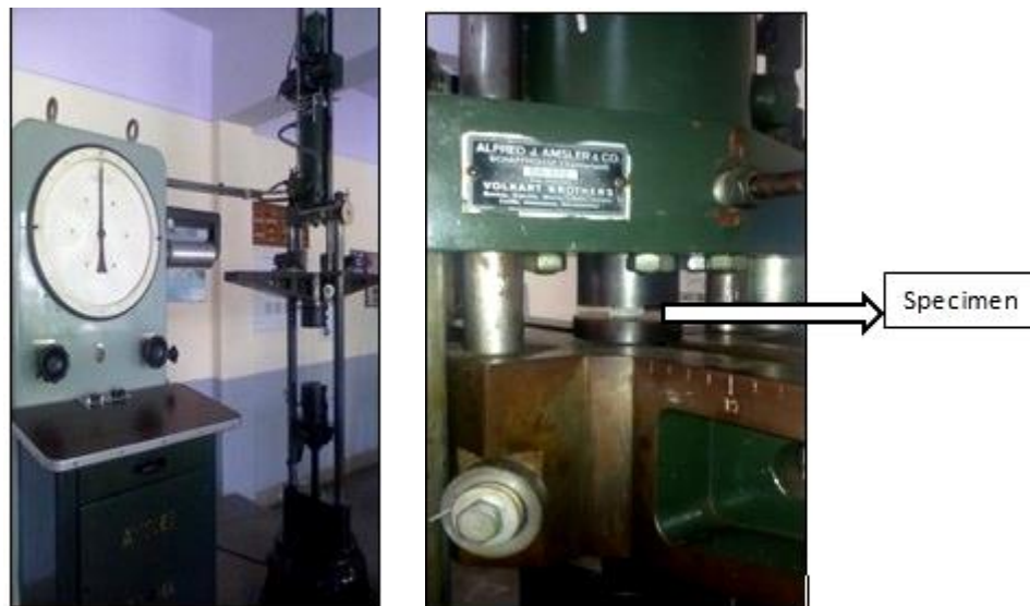
Fig. 3: Compression testing for GFRP and S-GFRP using UTM
