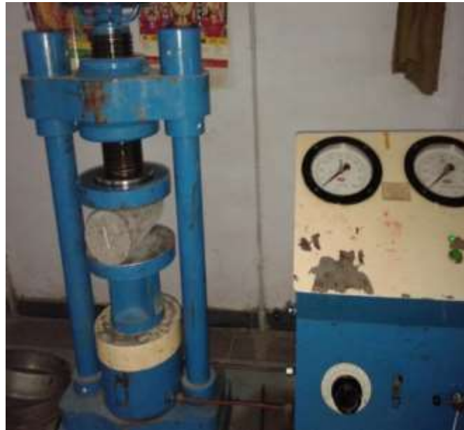
Fig. 11: Specimen loading for the split tensile strength test
