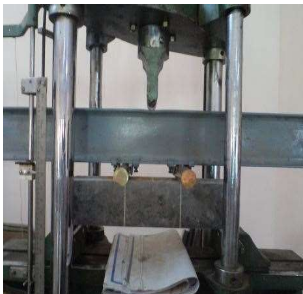
Fig. 3.10: Specimen loading for the flexural strength test
