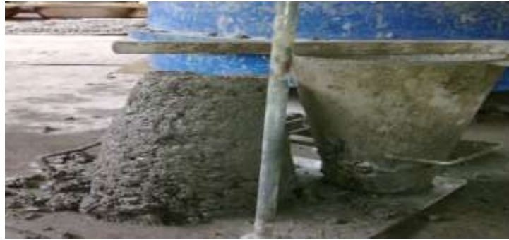
Fig. 6: Workability test conducted in the lab
