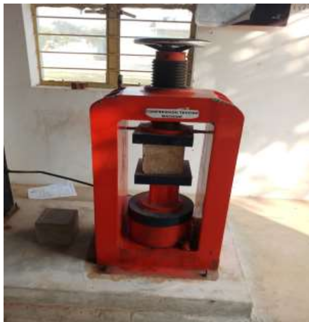
Fig. 7: Compressive strength test conducted in the lab
