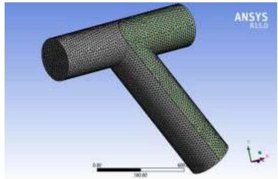
Fig. 10: Meshing view of modified model-I
