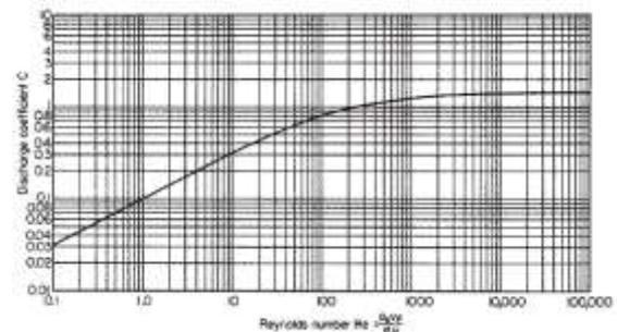
Fig. 1: Screen discharge coefficients, plain square-mesh screens. (Courtesy of E. I. du Pont de Nemours & Co.)
