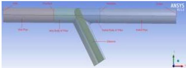
**Fig. 14: Illustration of boundaries and components of the modified model-II simulations**
