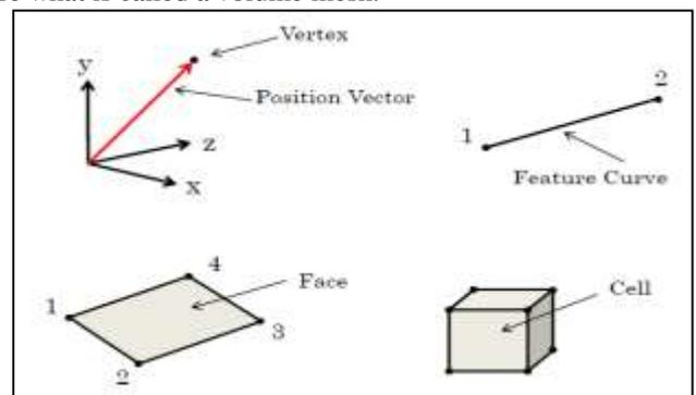
Fig. 7: Illustration of the individual components of a volume mesh
