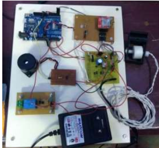
Fig. 3: Reed Switch interfaced with Arduino and GSM Module
