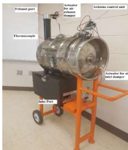
Fig. 5: Final product with main components labeled
