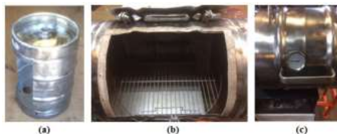
Fig. 3: (a) Smoker chamber with door opening and exhaust shown in the bottom, (b) finalized smoker with door hinged and leather insulation around the periphery, (c) smoker door closed with initial thermostat
