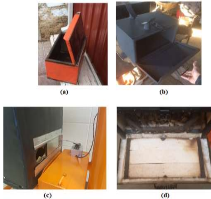
Fig. 4: Smoker box (a) cut from tools box, (b) paint removed and first coat of high temperature paint applied, (c) air inlet ports drilled and dampers installed with actuators connected to the Arduino, (d) high temperature ceramic insulation installed on the inner surface of the burner firebox
