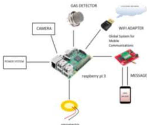
Fig. 1: System architecture (Camera, Gas detector, wifi Adapter will add for the future scope)
