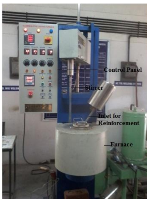
Fig. 1: Stir Casting Set up
