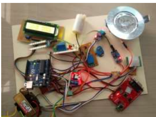
Fig. 4: Transmitter part of greenhouse monitoring and controlling system
