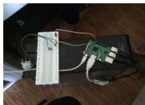
Fig. 5: Connections between Raspberry Pi, breadboard and PIR sensors
