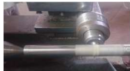
Fig7: Ball burnishing operation for EN24 Steel
