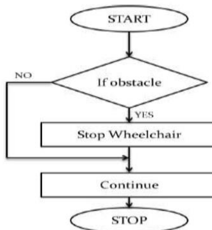
Fig 4. Flow chart of the obstacle sensor
