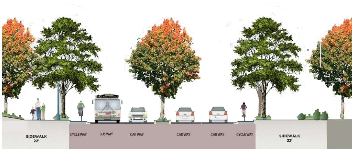
Figure 3. Section of all division of greenway showing sidewalk, cycleway, bus way and middle road divider
