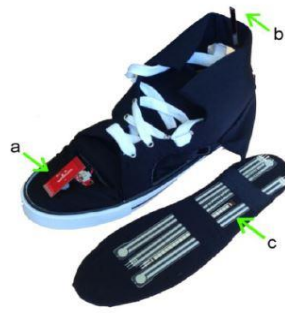
Fig.7: Instrument shoe (a) inertial measurement unit; (b) flexible goniometer; and (c) pressure sensors which are situated inside the insole.[9]
