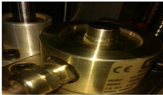
Figure4. Load Cell used in Slide Force Testing machine
