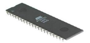
The AT89S52 is a high performance, low power consuming CMOS 8 bit microcontroller. This is manufactured using ATMEL's non-volatile & high density memory technology. Highly flexible in operation. The ATMEL AT89S52 have the following features:- 8K bytes of Flash, 256 Bytes of RAM, 32 I/O Lines, Watchdog timer, two data pointers,
