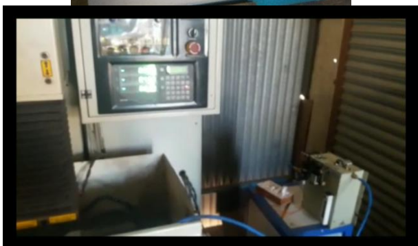
Figure: Setup of Near dry & dryEDM
