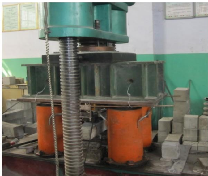
Fig.10. Testing apparatus of flexural toughness [13]
