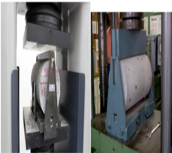
Fig.6. Tensile strength test on the cylindrical specimen
