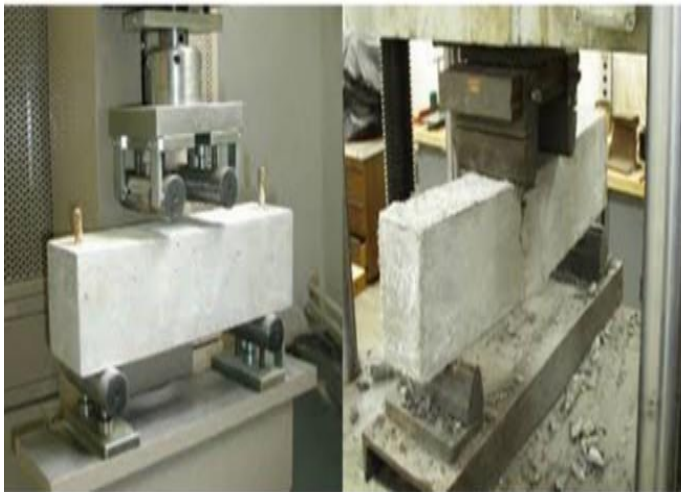
Fig.9. Flexural strength setup before testing
