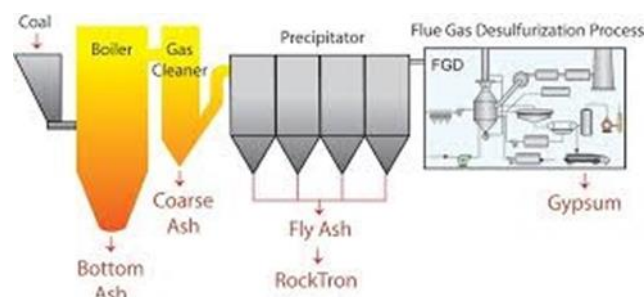
Fig.1. Collection of fly ash from exhaust gases by the electronic precipitator
