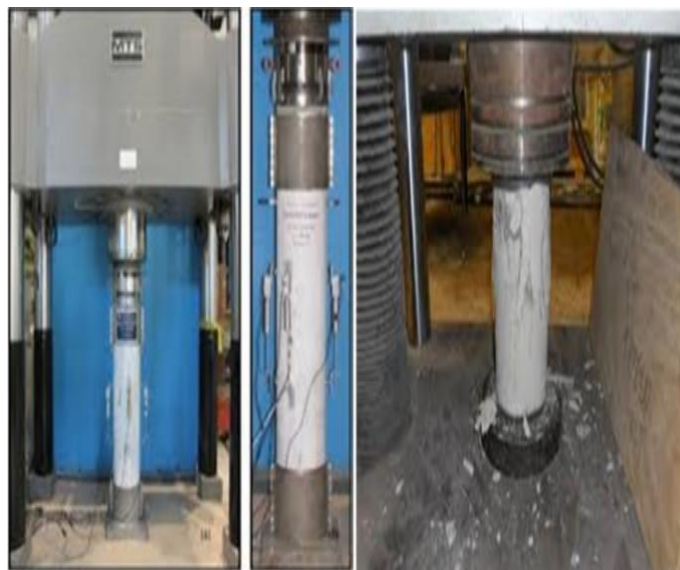
Fig.4. Crack pattern at ultimate failure load of cylindrical specimen
