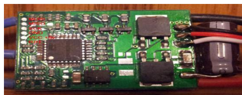
Fig 3: Internal Circuit of Electronic Speed Controller
