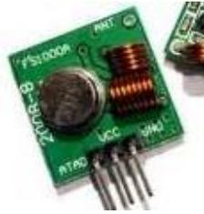
An RF transmitter module is a small PCB sub-assembly capable of transmitting a radio wave and modulating that wave to carry data. Transmitter modules are usually implemented alongside a micro controller which will provide data to the module which can be transmitted. RF transmitters are usually subject to regulatory requirements which dictate the maximum allowable transmitter power output, harmonics, and band edge requirements.
