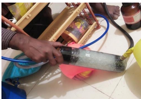
Fig 1.3 H2S Scrubber unit
