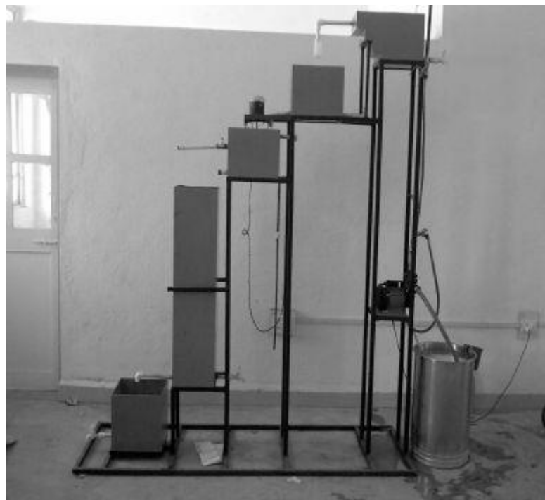
Figure- 4: Laboratory Scale grey water treatment plant
