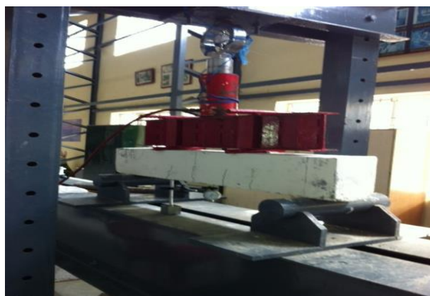
The fig-5 Crack pattern of PCS beams
