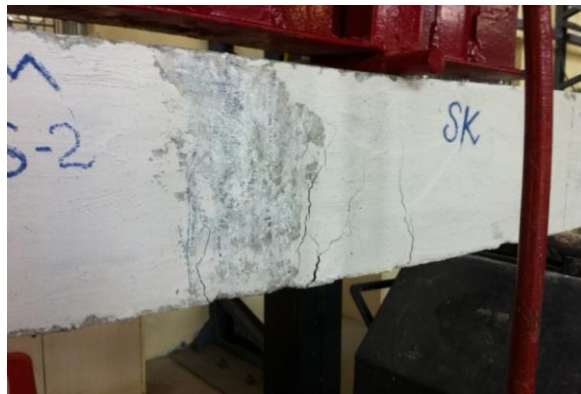
Fig-4 Crack Pattern
