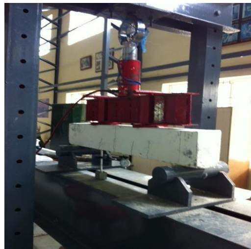
Fig-4 Test setup of beam
