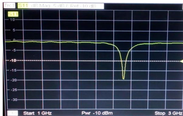
Fig.3.4.c. Measured Return Loss
