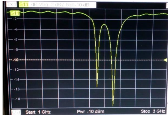
Fig.3.3.c. Measured Return Loss
