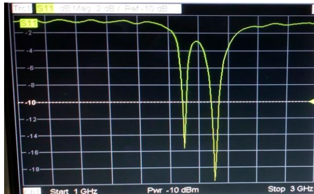
Fig.3.2.c. Measured Return Loss
