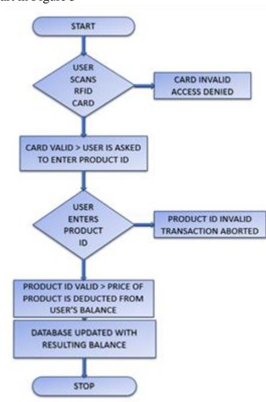
Figure 5: Transaction system flowchart
