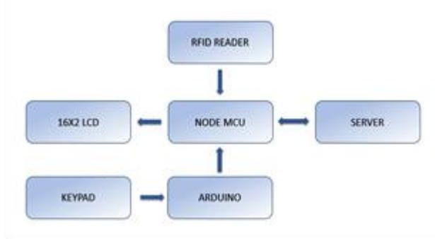
Figure 4: Transaction system block diagram
