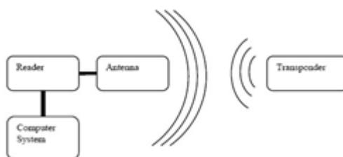
Figure 1: Basic RFID
