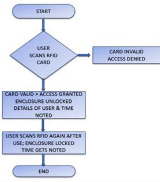
**Figure 3: Access control system flowchart**
