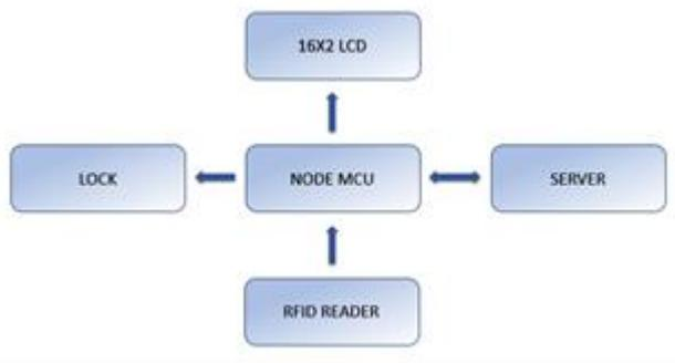
**Figure 2: Access control system block diagram**
