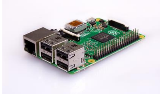
Fig 4: Raspberry Pi: A Single board computer used for purpose of experimentation for this project
