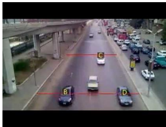
Fig 5: An image illustrating the two reference lines for calculation of speed.
