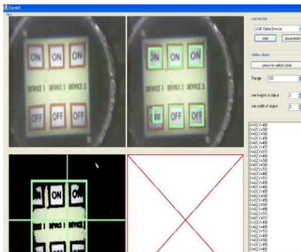
The virtual image is been projected and analyzed using a camera. We have developed a C++ program to analyze the image. We input a camera image as an input image then feature detection technique is used to find out the interesting point in an image and then extracted part is mapped as a viewing coordinate of a user with the addition of a virtual environment features.
