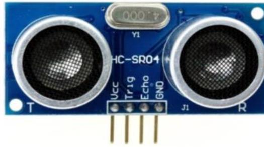
**Fig. 4 Ultrasonic Sensor**
