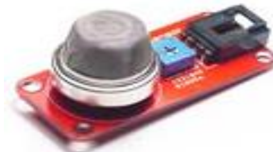
Fig.9 Gas Sensor Modules
