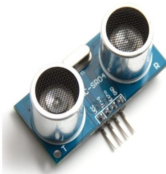
**Figure 1 Ultrasonic sensor**
