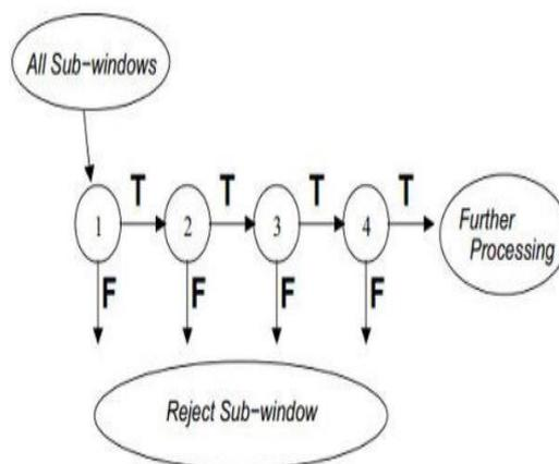
**Figure 4. Stages of the cascade classifier**
