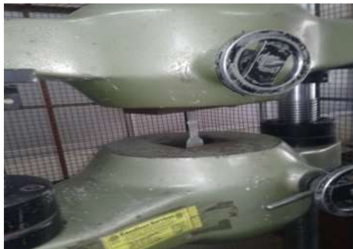
Fig. 3.9 Process Setup for Tensile Test
