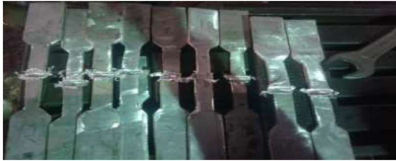
Fig. 3.8 Friction stir weld samples
