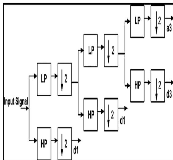
Fig. 4. Wavelet Transform Filter Structure Block Diagram
