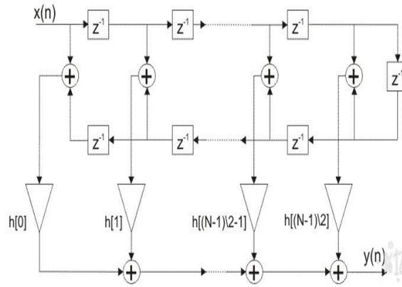
Fig 3. Linear Phase FIR Filter Design
