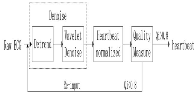
Fig 1. Existing ECG Signal Block Diagram
