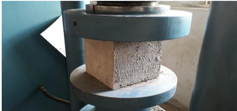
Fig. 2: Compressive Strength Test
