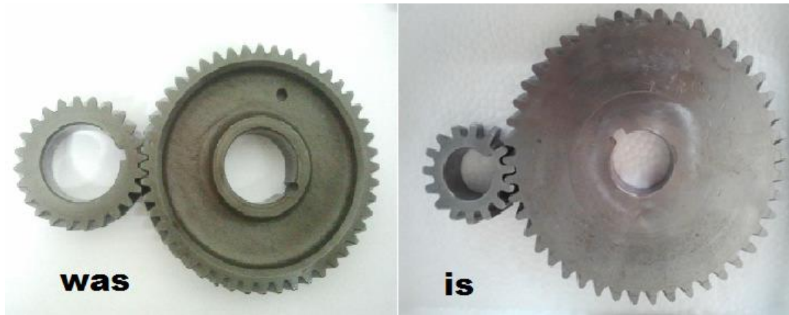
Fig. 5 Crankshaft to Camshaft Ratio Modification
