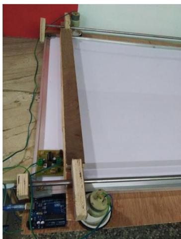
**Fig: 4 Controller, Motors and I293D Setup**
