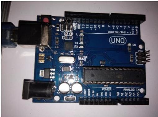
**Fig:-1. Arduino-Uno with ATMEGA-328P Microcontroller**
