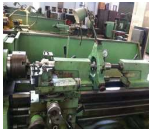
Figure 3.1: A Lathe Machine With A Setup Used For Experiment Figure 3.2: Joining of Specimen in Progress
