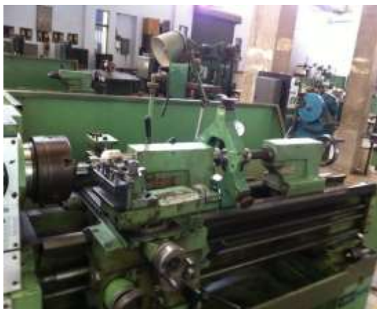
Figure 3.1: A Lathe Machine With A Setup Used For Experiment Figure 3.2: Joining of Specimen in Progress
