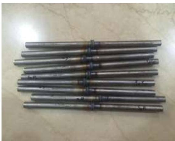
Figure 4.8 Samples of AISI 304 and AISI 4340 joined by RFW
