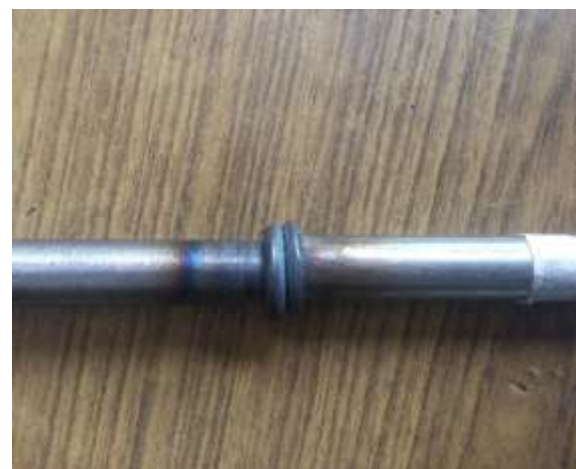
Figure 4.9 Joint-interface of AISI 304/434
