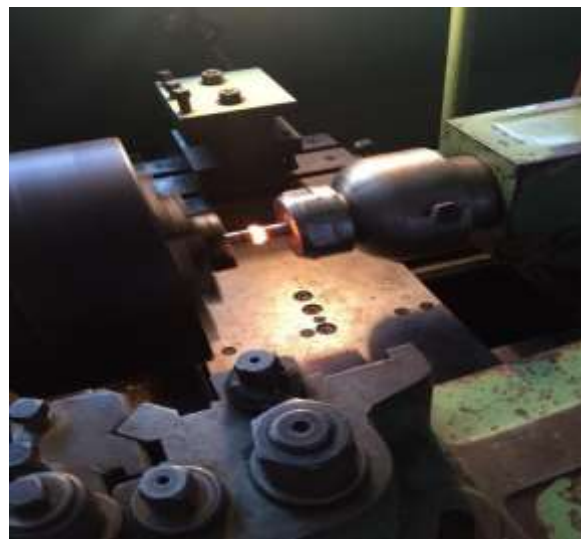
Fig 3.7 Joining of AISI304/4340 at Lathe Machine
