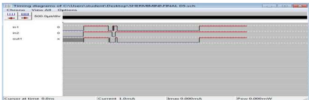
Fig. 9 Timing Diagram of the Proposed flip flop
